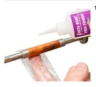
1. Turn the lathe on to about 500 RPM. Place a plastic bag on your finger, and apply a thin bead of CA Pen Finish onto the blank while spreading it across the blank with the plastic bag.
