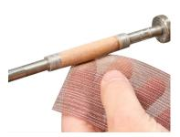
1. Turn the blank down to the desired shape and bushing diameter, then sand the blank through 400 grit. With a clean paper towel, remove all sanding dust.
