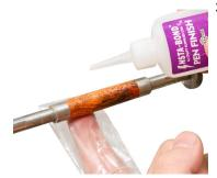
3. Repeat this process until you have 3 to 5 even coats of Insta-Bond™ CA Pen Finish. Note Do not sand between coats as this will result in a cloudy finish.
