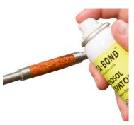
2. Lightly mist the blank with Insta-Bond™ Aerosol Activator to cure the CA.
