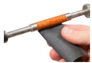
2. Once the blank is sanded, you can finish the CA Pen Finish using MicroMesh® Polishing Sheets. Wet sand the blank using grits 1500, 2400, 3600, 4000, 6000, 8000, & 12000.
