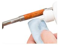
3. Once the blank is wet sanded and no scratch marks remain, polish the blank using 20/20 Plasti-Polish\*. Using a clean dry cloth apply a small amount of Plasti-Polish\* to the blank and buff until clean and dry.
