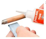
2. Using Insta-Bond™ Thin CA glue and paper towel, cover the blank with a thin coat of CA to seal and strengthen the wood. Spray the blank with Insta-Bond™ Aerosol Activator to cure the glue.
