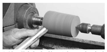
**1.** Select a block 3" x 3" x 4" long. A close-grained wood with straight grain through the stem is recommended. Mount the blank between centers on the lathe and turn it until round using a roughing gouge.
