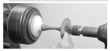
**11.** Turn the bottom of the stem until it's clean and smooth. Sand the base.
