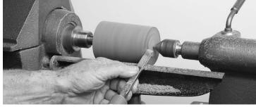
**2.** Square both ends of the blank using the long point of skew chisel flat on its side.
