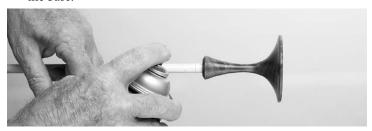
**12.** Using a wood dowel to hold the stem, apply a coat of Masters Magic (or similar) lacquer, wait a few minutes and apply a second coat.
