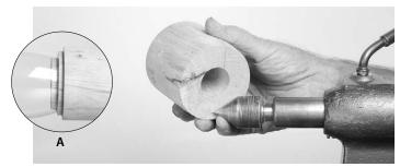
**13.** With the stem set aside to dry, turn a jig that will align and hold the glass in place while the adhesive cures. To do this, turn a cylinder 3 1/2" diameter by 4" long between centers. Drill a hole in one end of the cylinder to fit over the revolving center. Turn a tenon on the opposite end of the cylinder to fit snug inside the goblet opening (see figure A).
