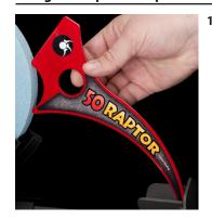
**1.** With the grinder completely stopped, place the end of the Raptor tool in the tool support arm as shown. Adjust the support arm as needed so that the two contact points on the Raptor tool contact the wheel face. Lock the support arm securely in place. Remove the Raptor tool.
