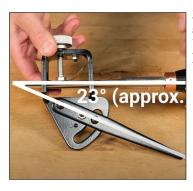
**2.** The leg angle needs to be set at approximately 23 Degrees. Use the top notch for to set the leg angle and lock in place.
