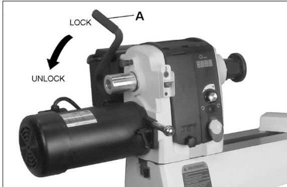
Figure 7-1: headstock movement
