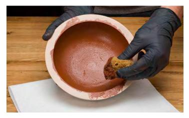
**4.** Once the first coat has dried for at least a 1/2 hour, apply the second coat of primer. Let the primer cure for at least 12 hours before applying Metal Effects Reactive Metal Paints.
