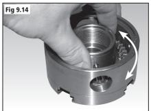
To check that the scroll gear has registered correctly with the jaw slides, move the scroll gear by hand whilst applying downwards pressure to it to observe the movement of the jaw slides. If additional pressure is required to move the jaw slides, hold the scroll gear in position by hand and turn it using the chuck key, **Fig 9.15**.
