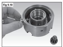
Carefully turn the chuck body to face upwards. This will allow the scroll gear to drop from the chuck body. Ensure it is caught to prevent any damage, **Fig 9.11**.
