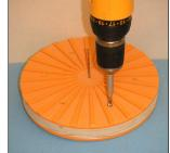
For the required stiffness, attach the SegEasy plate to a 3/4" thick piece of MDF or plywood cut to the same diameter as the plate. Use #6 x 3/4" flat-head wood screws to attach the plate to the MDF..
