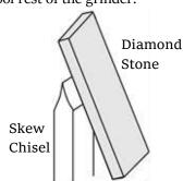
Then place the stone on the flat edge behind the long point of the skew. Hone this area with the same back and forth motion, being sure to keep the stone flat on this surface. Finally, hone the area behind the short point in a similar fashion - even though that section has been rounded all the way to the ferrule, you can still refine the short point by keeping the
