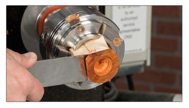
**9.** Lightly coat the inside of the ring blank with thick or flexible CA glue or Epoxy and insert the ring core. Wipe away any excess glue.
