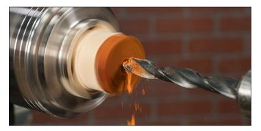
**6.** Now with a skew or narrow scraper flat on its side open up the drilled hole until the ring core fits in the hole. We recommend testing the fit frequently to avoid an oversized hole. Ideally the ring core should just barely fit in the hole. *Hint: We recommend having a few different sizes of ring cores on hand in case you make the hole too large, then you can simply go to the next size up and salvage the blank.*
