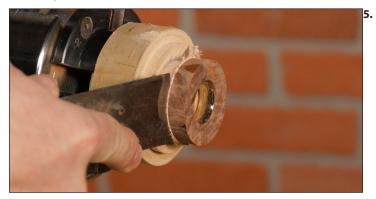
Lightly coat the inside of the ring blank with thick or flexible CA glue or Epoxy and insert the ring core. Wipe away any excess glue.
