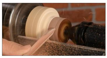
**5.** Select a drill bit half the diameter of the ring you are turning. Mount the drill bit in a drill chuck and drill through the ring blank.
