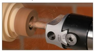
**4.** Repeat this process until you are close to having the ring core fit. Test the fit of your ring core frequently with the lathe off, careful not to oversize the hole. The boring head allows very precise cuts, take your time and make light cuts until the core fits perfectly.
