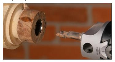
**5.** Remove the ring blank from the waste block. Slowly pry the blank from the waste block using a putty knife and it will release the ring blank. **Do not use too much pressure or the ring blank will break in half.**
