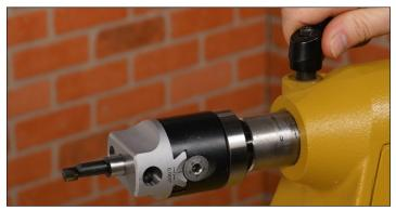
**3.** Bring up the tailstock until the cutter is close to the ring blank. Use the allen wrench and turn the dial counter-clockwise to move the cutter. Stop once the cutting edge is positioned to take a 1/8" cut. Turn the lathe on to around 2500 rpm and advance the boring head slowly until completely through the ring blank. Back out the boring head and adjust the dial to take another 1/8" pass. Do not take a cut wider than 3/16". If it starts to chatter, stop and take a narrower cut.
