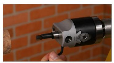
**2.** In order for the boring head to cut accurately the tailstock quill needs to be under tension. Slightly tighten the quill lock handle until there is a bit of resistance when advancing the quill. Your boring head is now ready to use.
