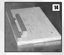
This is the jig I use to flex the body of the knife so the handle will be good and tight. If the blade is loose, it's worthless!
