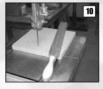
A small piece of scrap stock is used to elevate the knife to compensate for the thicker handle.
