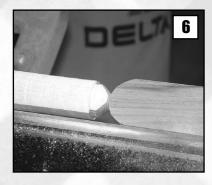
Form the transition between the blade and the handle. A half-bead and a chamfer work great to join these two elements.
