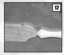
A 3/16" roundover bit in a laminate trimmer is used to ease the top of the curve. You won't be able to get in tight by the transition corner.
