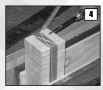
Find the center of the middle block on the handle side and carefully centerpunch it with a sharp awl. Do the same to the other end as well.
