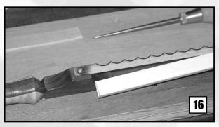
The plastic spline from a term paper cover is used for a guard. The guard should be placed over the back edge of the blade. If you try to put it over the teeth of the blade, it will get stuck.
