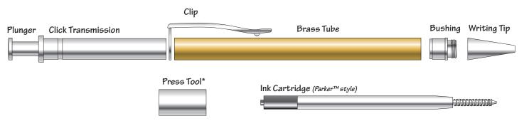
\*Press Tool for assembly only. Not a part of completed pen.
