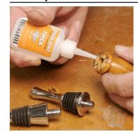
**1.** Remove the finished stopper from the mandrel. Place a few drops of Thick CA glue or 5 minute Epoxy into the threaded hole of the finished stopper. Screw the finished stopper onto the threaded stud of the bottle stopper. Make sure the turned stopper seats firmly against the stopper for a proper fit.
