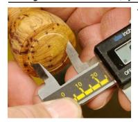
**1.** Use as set of calipers to measure the diameter of the insert. Scribe the end of the stopper using the sharp points of the caliper to indicate the diameter of the recess required for fitting the insert. *Hint*: When scribing the stopper, do so with the lathe turning at a slow speed to prevent a catch.
