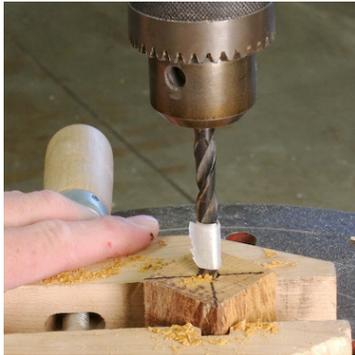
2. Center mark and drill a 11/32" diameter hole about 5/8" deep in the end of the blank. Make sure the drill bit is properly positioned at 90 degrees to the end of the blank prior to drilling so that the blank seats flat against the mandrel face. *Hint: Wrap masking tape around the drill bit to act as a depth gauge.*
