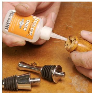
1. Remove the finished stopper from the mandrel. Place a few drops of Thick CA glue or 5 minute Epoxy into the threaded hole of the finished stopper. Screw the finished stopper onto the threaded stud of the bottle stopper. Make sure the turned stopper seats firmly against the stopper for a proper fit.
