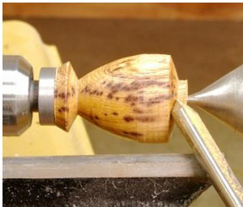
5. Turn the blank to shape with the revolving center supporting the work piece. Sand and finish the stopper. Slide the tailstock out of the way to sand and finish the end of the blank. Remove the revolving center and gently turn away the nub left by the revolving center. Sand and finish.
