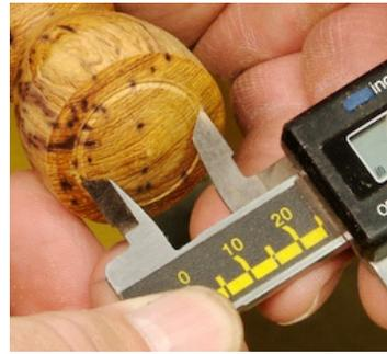
1. Use a set of calipers to measure the diameter of the insert. Scribe the end of the stopper using the sharp points of the caliper to indicate the diameter of the recess required for fitting the insert. *Hint: When scribing the stopper, do so with the lathe turning at a slow speed to prevent a catch.*
