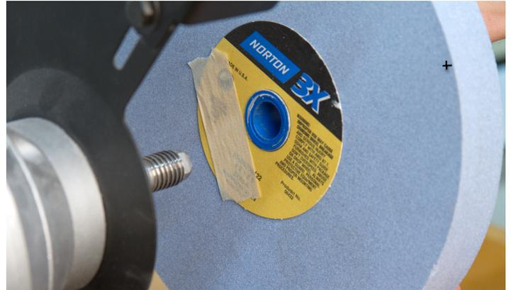
5. Reinstall the right side washer and tightening nut and tighten.
