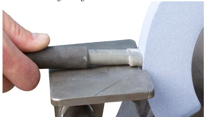
4. Continue to dress the wheel until all high points on the wheel have been ground down and the dresser fully engages the entire surface of the wheel. Move the wheel dresser side to side until the face of the wheel runs true. *Hint: Do not forcefully push the dresser into the wheel's surface. Doing so will cut the softer portions of the wheel much faster than the harder portions, adversely changing the shape of the wheel.*
