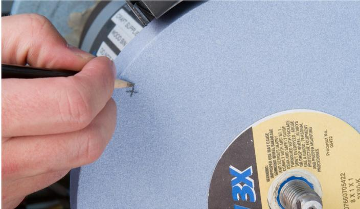
3. Place a single layer of masking tape on the paper washer on the right side of the wheel as shown. The tape should be positioned on the paper washer so that it is in line with the mark on the wheel and the center of the arbor.
