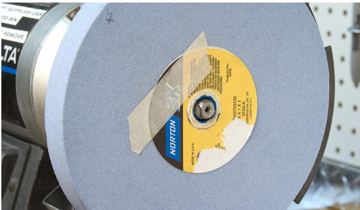
4. Place a single layer of tape on the paper washer on left side of the wheel with the tape positioned opposite the tape on the right side paper washer. Example: If the tape on the right side of the wheel is at 10 o'clock, the tape on the left side of the wheel should be located in the 8 o'clock position. If done properly, the tape on opposing sides of the wheel are positioned 180 degrees from one another.
