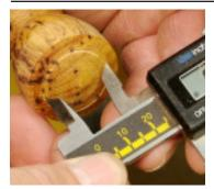
1. Use as set of calipers to measure the diameter of the insert. Scribe the end of the stopper using the sharp points of the caliper to indicate the diameter of the recess required for fitting the insert. *Hint*: When scribing the stopper, do so with the lathe turning at a slow speed to prevent a catch.
