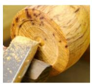
**2.** Turn the recess to the proper diameter and depth. Be sure to check for fit often to avoid turning an oversize recess.
