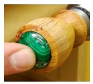
**3.** Using a flexible instant glue or RTV silicone adhesive, place a small amount of adhesive in the recess and press the insert firmly into place.
