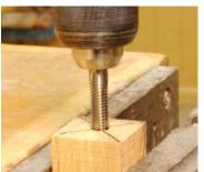
**3.** Clamp the blank securely in a bench vise. Using a 3/8"-16 tpi drill tap in a variable speed drill, tap the hole in the blank. Go slowly.
