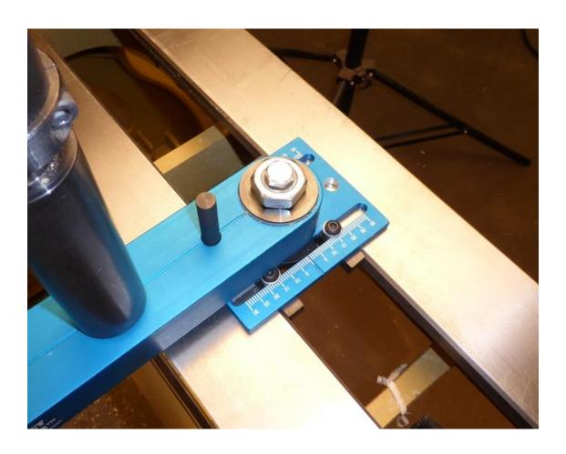
6. Adjust the height of the Cutting Head (8) so the #4 Hunter Cutter (6) is centered on the lathe centerline or spindle. It is helpful to install a spur center or other accessory that has a point on the centerline or center of the lathe to align the #4 Hunter Cutter (6) to the center of the lathe. Once the #4 Hunter Cutter (6) is centered on the lathe centerline, lock the Cutting Head (8) in place with the Cutting Head Locking Knob (5).
