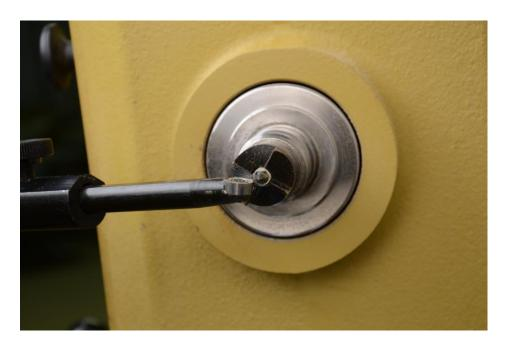
7. Slide the Locating Collar (9) which was mounted on the Riser Post (10) earlier, up to the bottom of the Cutting Head (8) and lock in place. This will allow the Cutting Head (8) to always return to the same height and will not need to be adjusted again.
