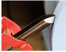
3. With the grinding wheel stationary, position the tool holder in the sharpening jig slide. With the tool in the upright position, place the bevel of the set up tool against the face of the wheel. Adjust the slide in or out as needed until the bevel of the set up tool rests flat against the wheel face.
