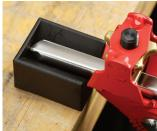
2. Clamp the set up tool in the tool holder with 2" protruding beyond the front of the tool holder. This can be done using a measuring tape or the Jamieson Grinding Jig Guide that mounts on a workbench top for easy set up. Note: When setting up for the "Irish" grind, 2 1/8" of tool must protrude beyond the front of the tool holder.
