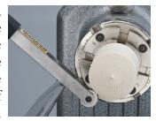
with the wheel contacting the work at about a 7–8 o'clock position on the work. This leveraging action creates far more pressure than the standard method of holding the texturing tool. Note- be careful not to create too much pressure as it may force the work out of the chuck.
